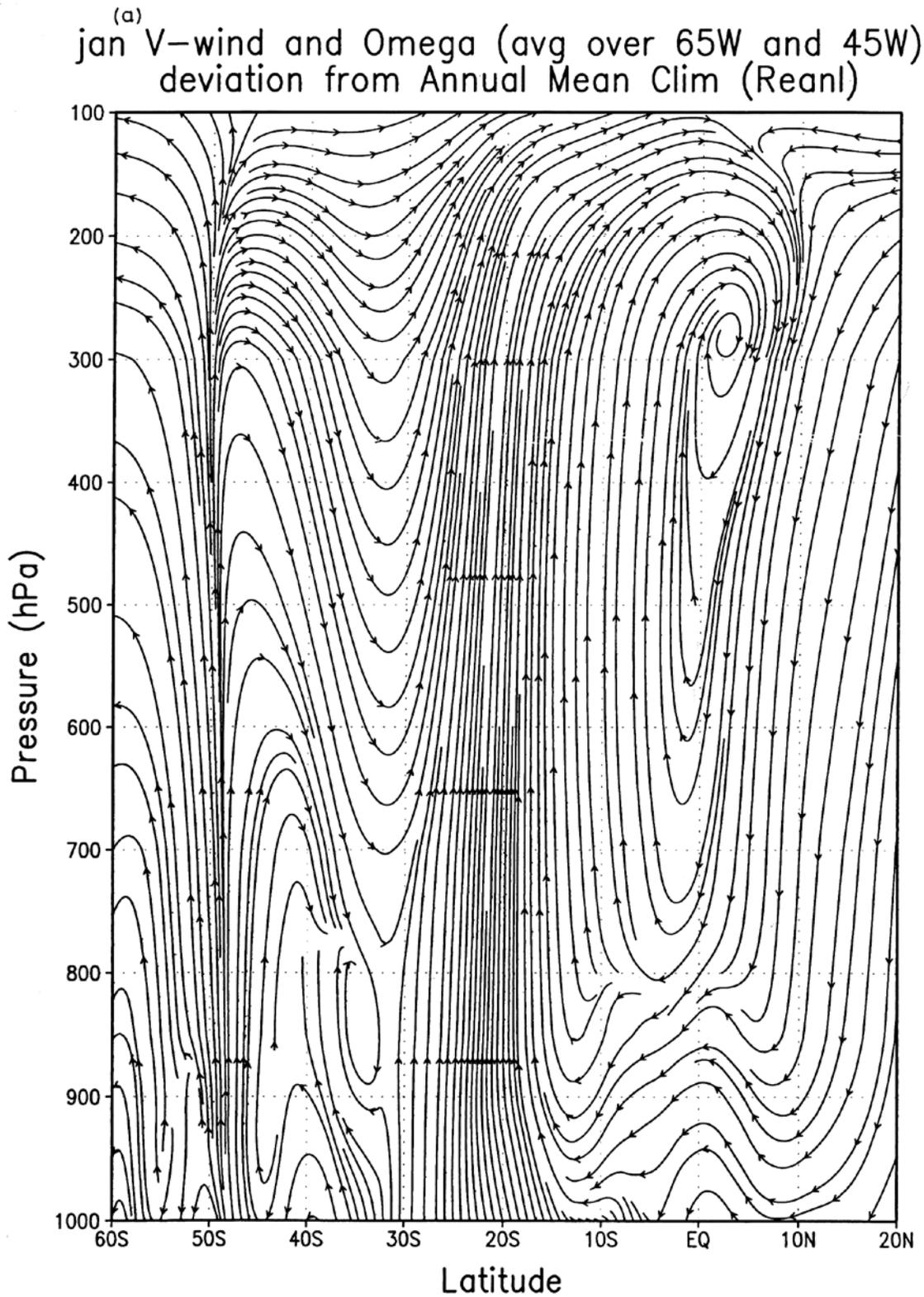
Fig. 10(a). Zonally-averaged meridional-vertical circulation over South America : January (Dec, Jan, Feb)
