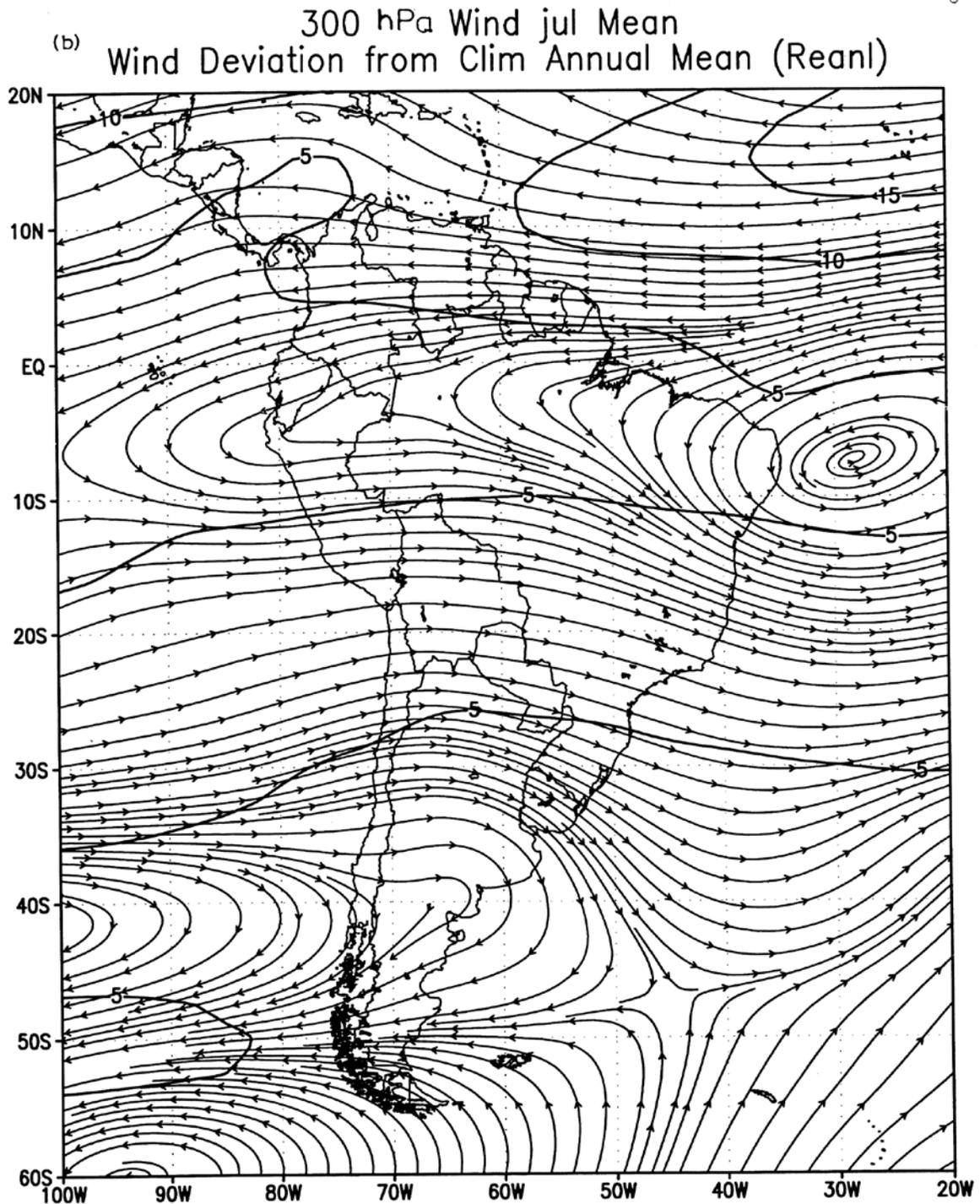
Fig. 9(b). Monsoonal (deviation of observed monthly mean from the mean annual mean) wind field over South America and surrounding oceans in July at 300 hPa
