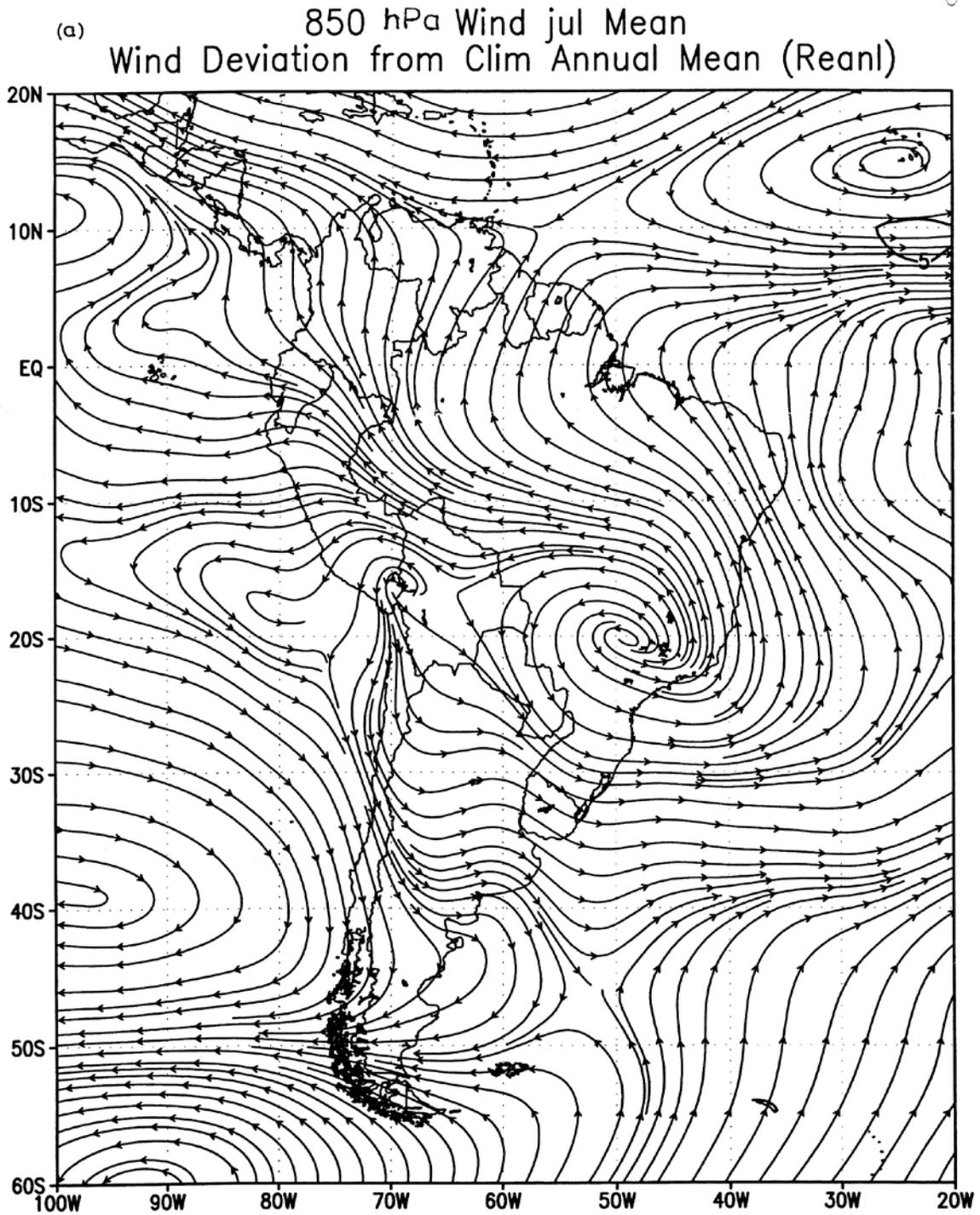
Fig. 9(a). Monsoonal (deviation of observed monthly mean from the mean annual mean) wind field over South America and surrounding oceans in July at 850 hPa
