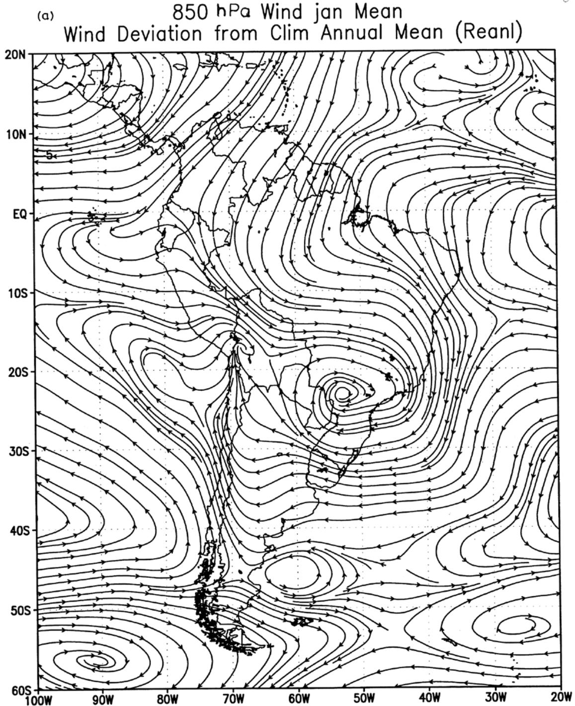
Fig. 8(a). Monsoonal (deviation of observed monthly mean from the annual mean) wind field over South America and surrounding oceans in January at 850 hPa
