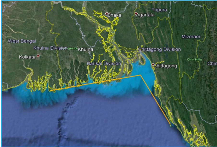
Fig. 2. Filter used in the creation of synthetic tracks affecting Bangladesh. The centers of all the simulated tropical cyclones passed over one (or possibly both) of the two line segments shown in orange. Rainfall was calculated at Dhaka, at center near the top of the map
