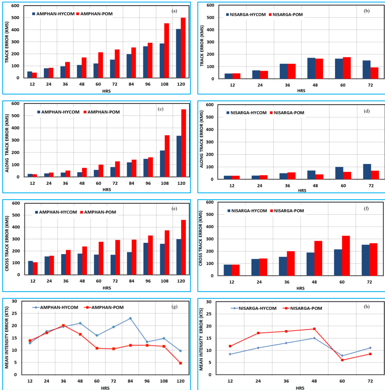
Figs. 9(a-h). Mean values of DPE, ATE, CTE (in Kilometers) and absolute intensity error (in Knots) of HPOM and HCOM forecasts in (a), (c), (e) & (g) for AMPHAN and in (b), (d), (f) & (h) for Nisarga respectively
