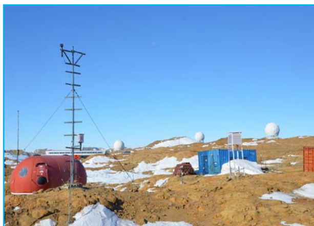
Fig. 1. Current weather instruments system, solar radiation sensors and surface observatory installed near Bharati station, Antarctica
