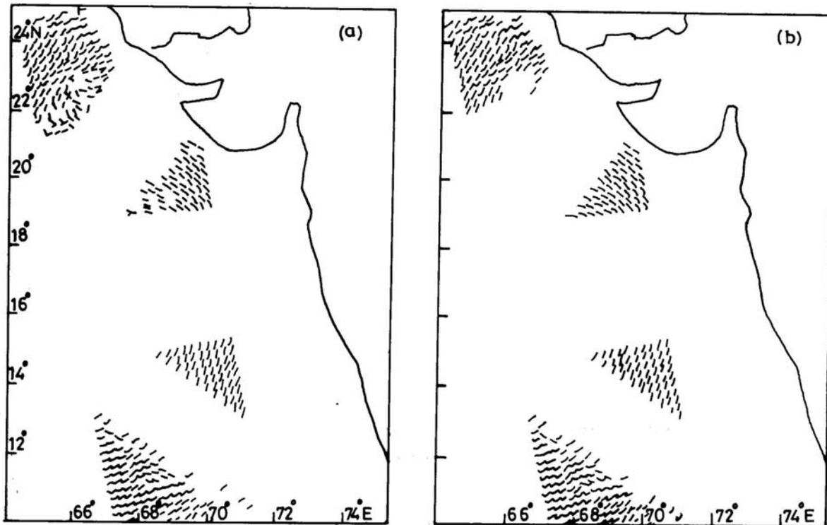
**Figs. 3(a&b).** (a) ERS-2 scatterometer wind data as received at NCMRWF (pass over Arabian sea) Date : 1800 UTC, 7 June 1998, (b) ERS-2 scatterometer wind data after quality control (pass over Arabian sea) Date :1800 UTC, 7 June 1998
