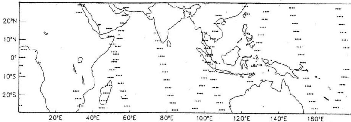
Fig. 4(c). Availability of ERS-2 wind data at NCMRWF (along the satellite track) Date : 8 June 1998
