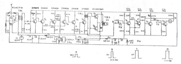
Fig. 1. 401 MHz receiver for testing radiosonde
