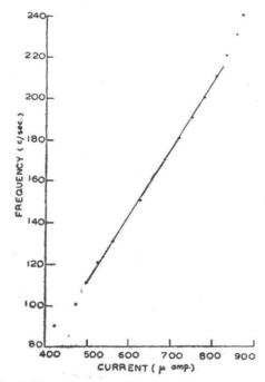
Fig. 2. Linear relationship between current and frequency
