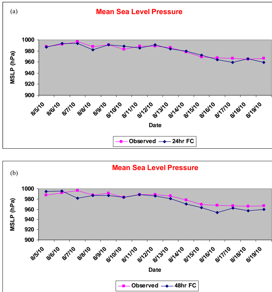
Figs. 16(a&b). (a) An inter-comparison of daily 24 hours forecast mean sea level pressure of 0000 UTC and corresponding observed mean sea level pressure of Maitri during 5 August 2010 to 19 August 2010 and (b) same as (a) except for the 48 hours forecast
