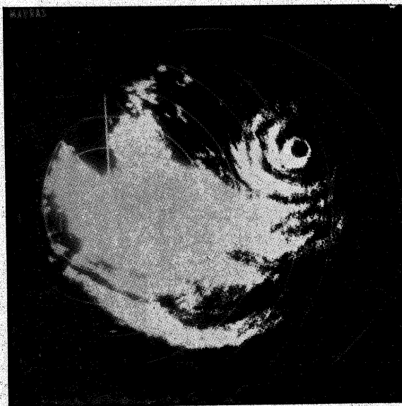
Fig. 6. Off centred PPI picture at 1225 IST of 11 May showing complete eye at a range of about 260 km. Markers are at 40 km intervals
