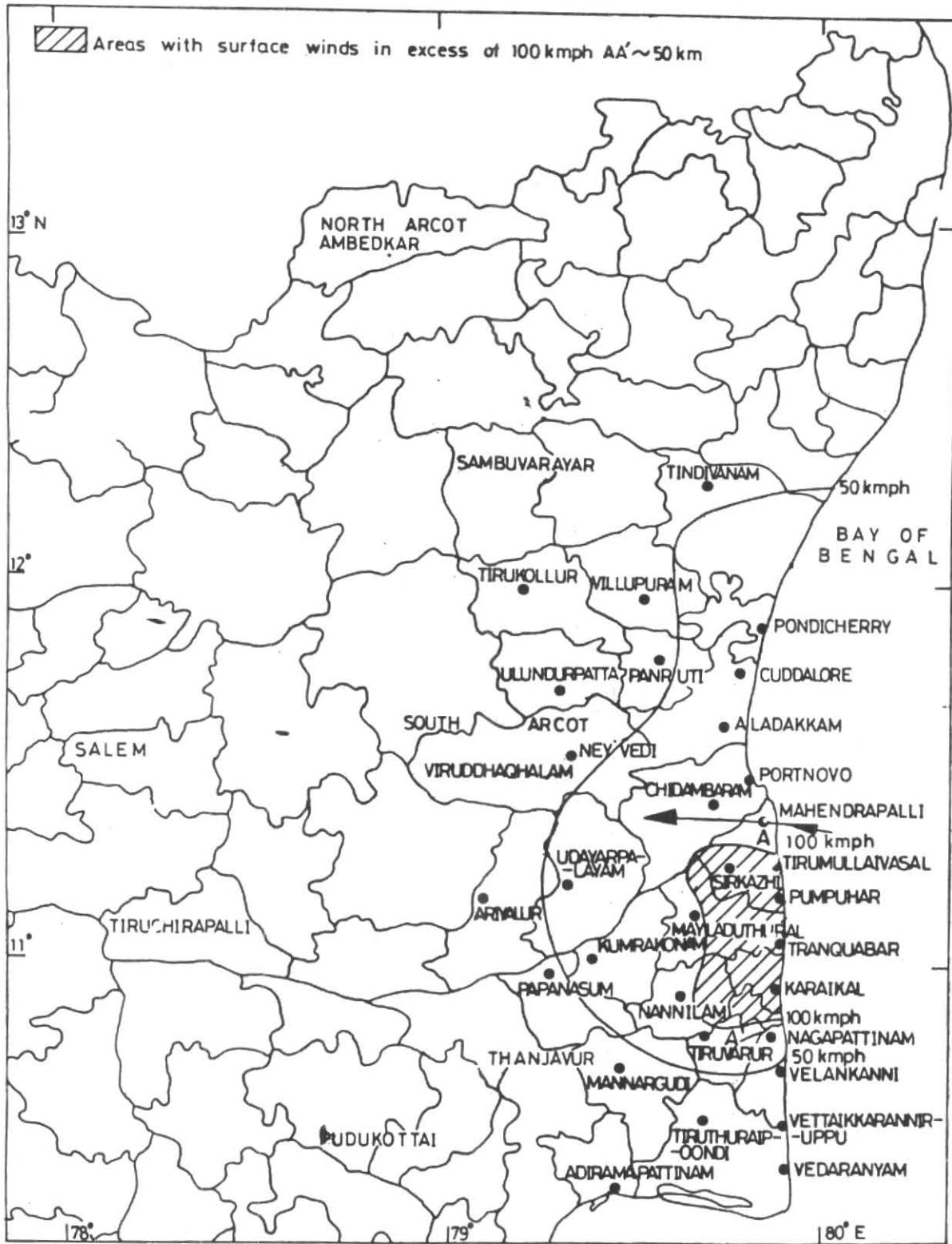
Fig. 2. Estimated/Observed surface winds in the area close to storm track as revealed by post cyclone-survey
