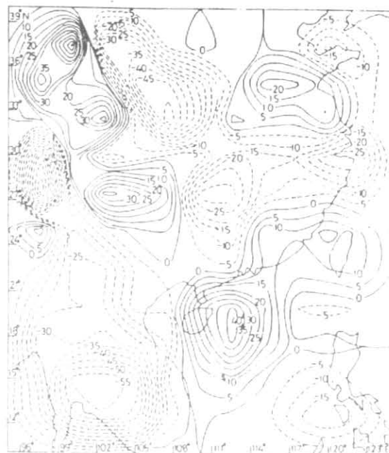
Fig.5. Distribution of vertical velocity (unit: 10^{-4} hPa s^{-1} ) at 500 hPa at 1200 UTC on 1 July 1979. Positive denotes downward and negative upward.
