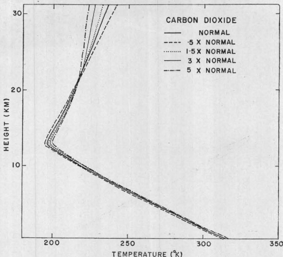
Fig. 6. Radiative equilibrium temperature for given changes in the mixing ratio of carbon dioxide
