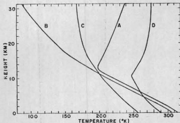
Fig. 3. Radiative equilibrium temperature obtained for (A) normal atmosphere (B) Water vapour atmosphere (C) Carbon dioxide atmosphere and (D) Ozone atmosphere
