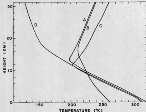
Fig. 4. Radiative equilibrium temperature, obtained for (A) Normal atmosphere (B) Water vapour absent (C) Carbon dioxide absent and (D) Ozone absent
