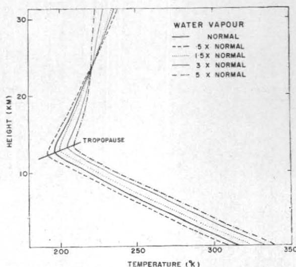
Fig. 5. Radiative equilibrium temperature for given changes in the mixing ratio of water vapour
