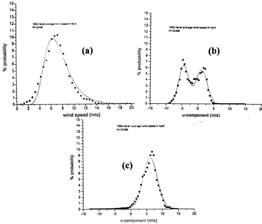
Fig. 1. (a) Weibull distribution of peak wind speed, (b&c) Gaussian distribution of wind component ( $u, v$ ) in April at 100m level
