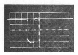
Fig. 3(b). Output of the blocking oscillator
