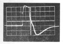
Fig. 3(a). Output of the pulse transformer
