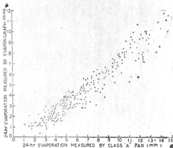
Fig. 5. Scatter diagram showing nature of relationship between daily measurements by Evaporigraph and Class A Pan in 1970
