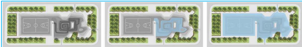
Fig. 15. Top view of the pilot water square - during dry periods, medium rain, and heavy storms (left to right)
