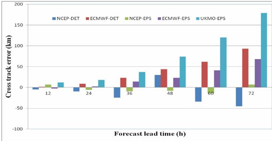
Fig. 8. Mean cross track (CT) position error bias based on NCEP, ECMWF deterministic and NCEP, ECMWF and UKMO ensemble forecast over North Indian Ocean (NIO)
