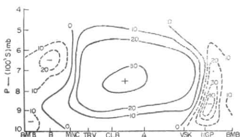
Fig. 13. Vertical profile of the deviations of specific humidity ( q ) from the mean (in tenths of gm/kg) around the boundary — 21 October 1963 (1200 GMT)
