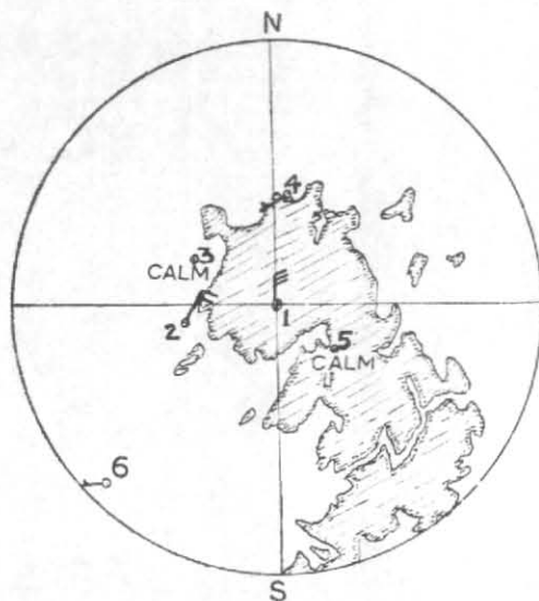
Fig. 8. Asymmetric distribution of winds — Safdarjung radar PPI Date — 4 August 1961, Time — 1413 IST, Radius — 15 miles Elevation — 3°, Movement of cloud — N to S
