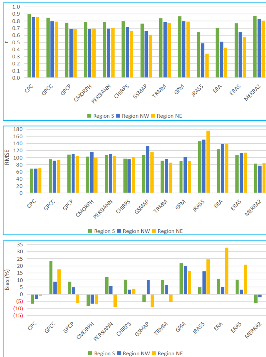
Fig. 4. The mean values of coefficient correlation, RMSE and bias (error) at three regional clusters for all months at monthly timescales
