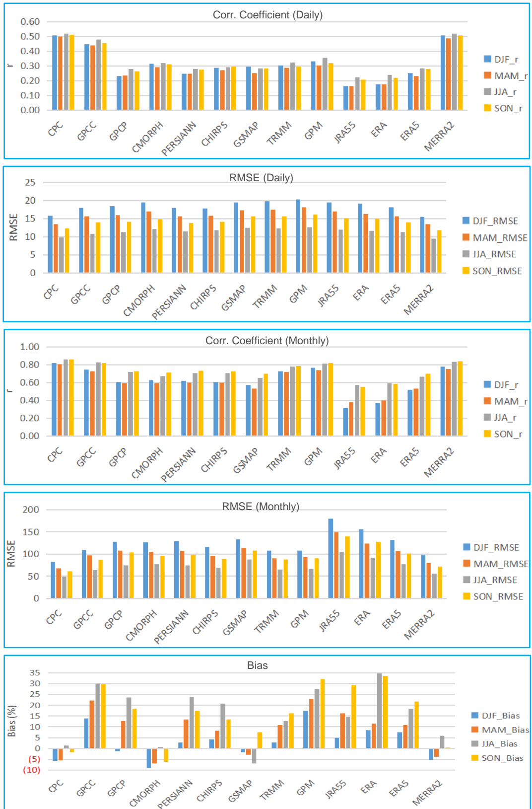
Fig. 3. The seasonal mean values of coefficient correlation, RMSE and bias (error) from all observation stations at daily and monthly timescales
