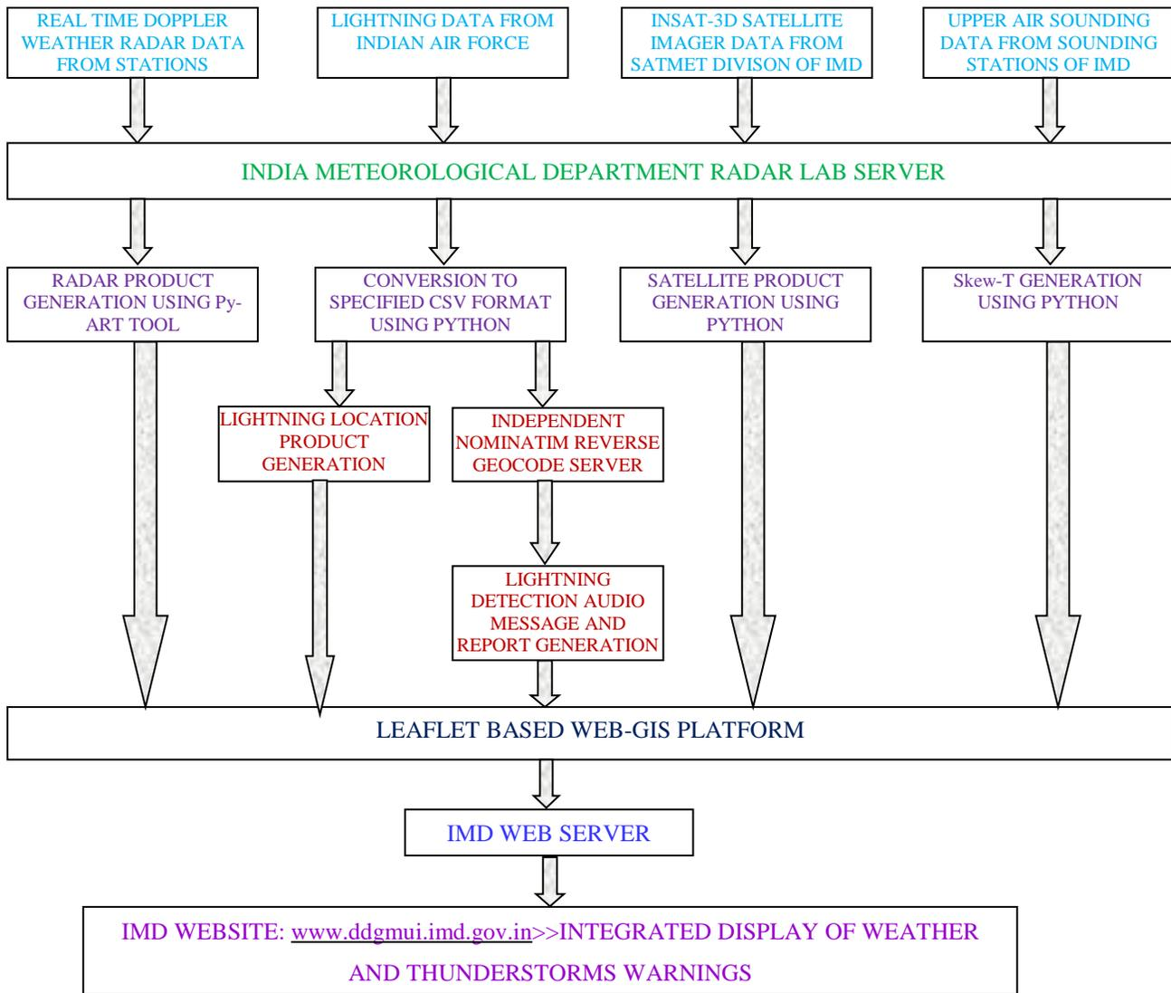
Fig. 3. Flow diagram of the development of a web-based Tool
