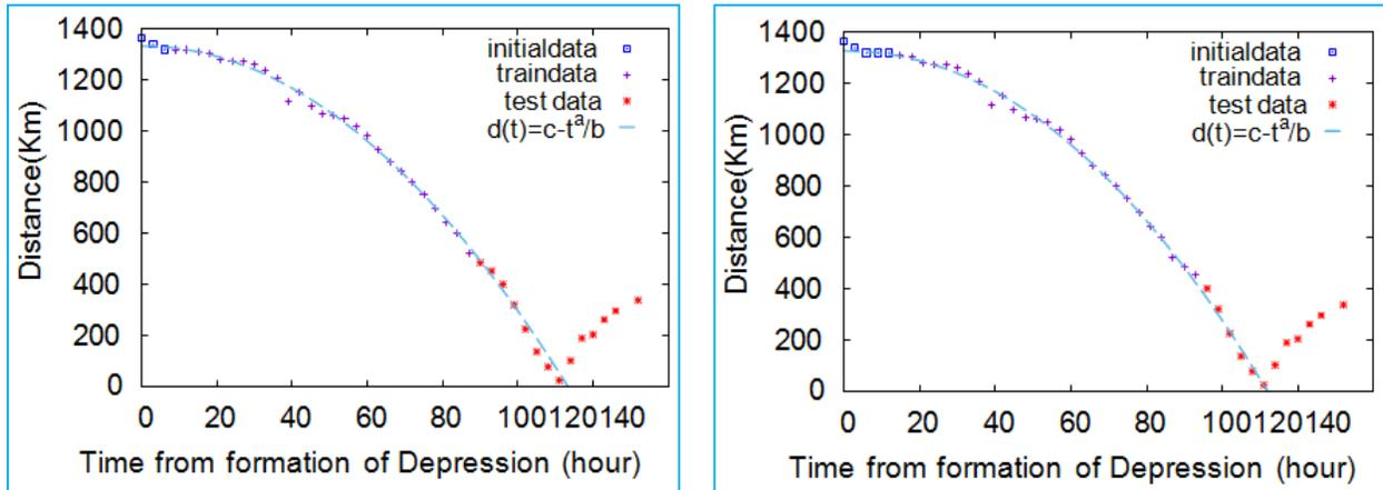
Fig. 4. Left : Curve fitting and prediction of the distance of the cyclone center from Kolkata with a lead time of upto 24 hours using data for the variation of distance with time; Right : Similar fitting and prediction with a lead time of up to 18 hours
