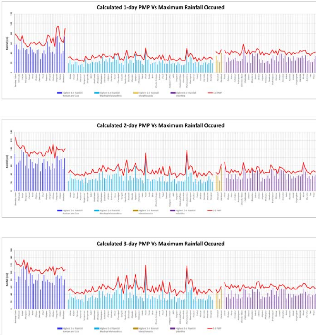
Fig. 4. 1-day, 2-day and 3-day PMP with maximum 1-day, 2-day & 3-day rainfall in 113 years
