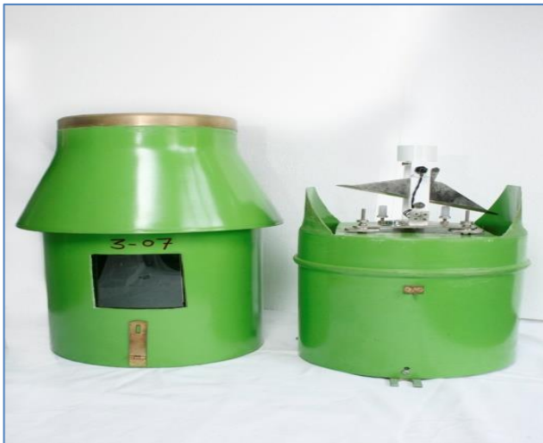
Fig.18 Tipping Bucket Rain-gauge sensor manufactured in workshop
