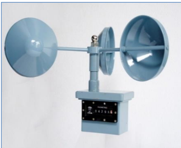
Fig. 19. Cup Counter Anemometer sensor manufactured in workshop
