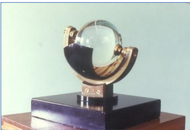
Fig. 25. Sunshine duration sensor manufactured in workshop
