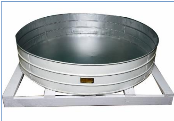
Fig. 24. Open-Pan-Evaporimeter sensor manufactured in workshop
