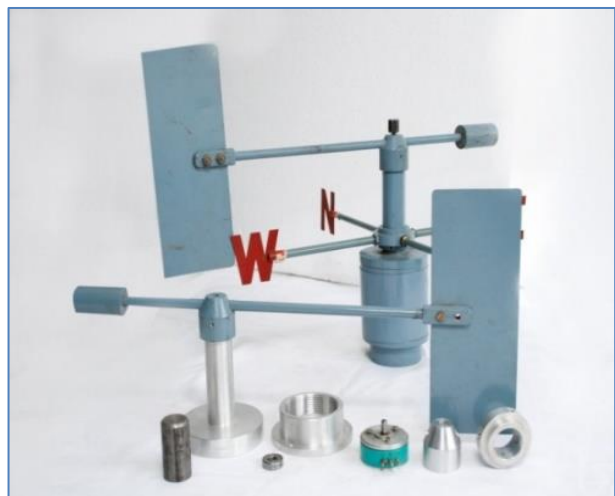
Fig. 21. Wind Direction sensor (Automatic), manufactured in workshop
