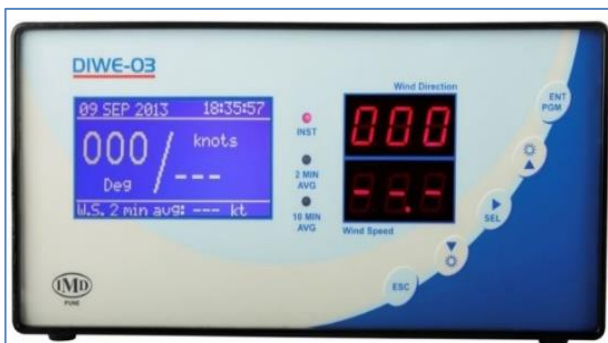
Fig. 30. Indigenously developed DIWE (WD/WS) developed system
