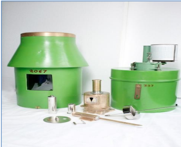
Fig. 17. Self-Recording Rain-gauge sensor manufactured in workshop
