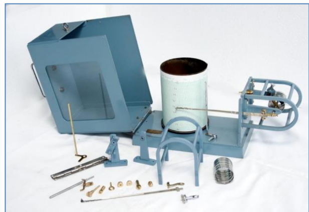
Fig. 15. Thermograph sensor manufactured in workshop
