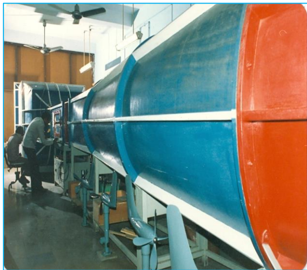
Fig. 14. Wind tunnel for the calibration of wind anemometer
