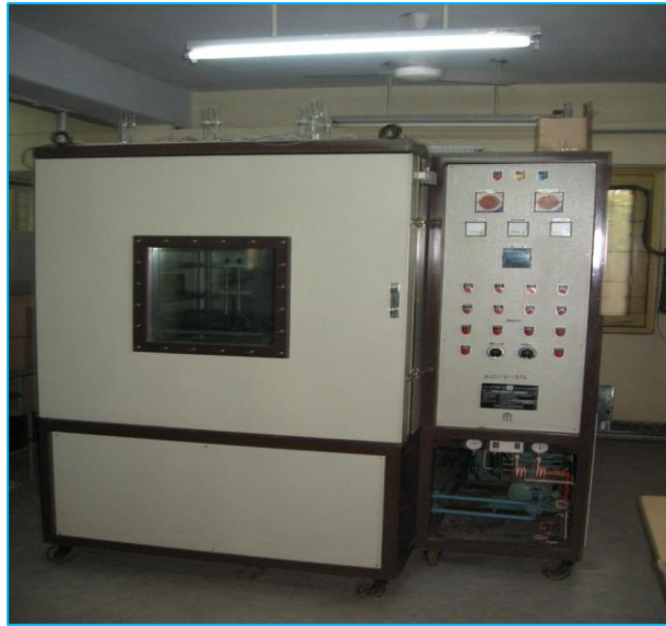
Fig. 13. Thermometer (digital) calibration chamber
