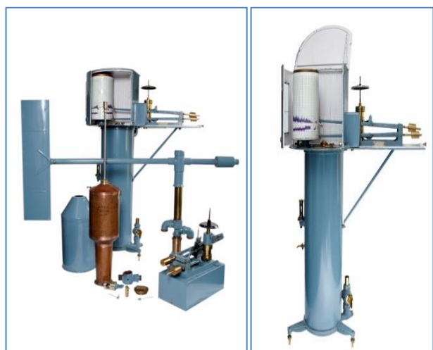
Fig. 22. Dynes Pressure Tube Anemograph sensor manufactured in workshop
