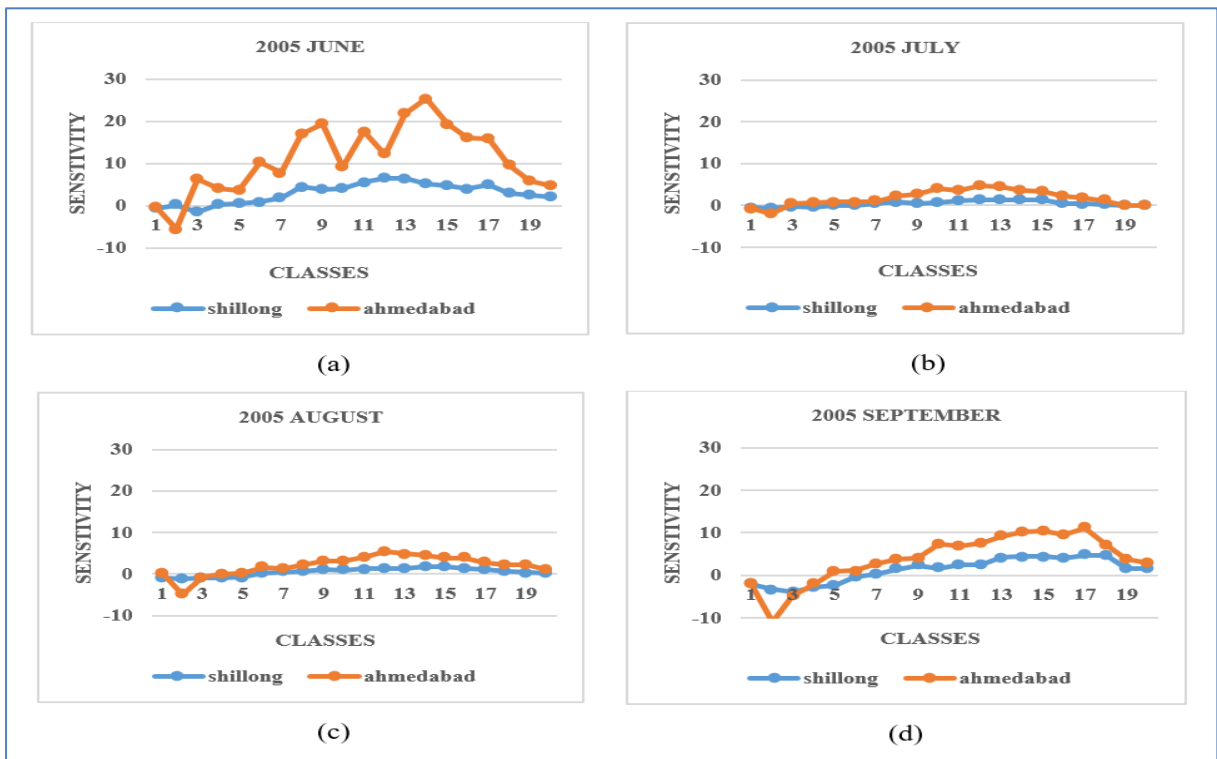
Fig. 8. Visualization of Sensitivity: Exploring the Relationship Between Pre-defined Disdrometer Drop Size Classes and Rainfall Rate.
