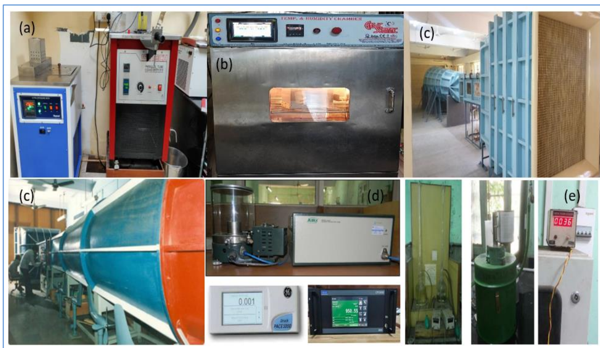
Figs. 2(a-e). (a) Ultra-cryogenic bath for calibration of all type of thermometers, (b) Temperature and Humidity chamber (c) and (d) Wind Tunnel for wind speed measurement calibration and testing, environmental chamber for calibration of AT/RH sensors, Thermographs and Hygrographs (e) Druck and Mensor pressure standards for calibration of all types of pressure sensors (f) Burret, pulse counter and dispenser for calibration of all types of rain measuring instruments and Tipping Bucket Rain Gauges
