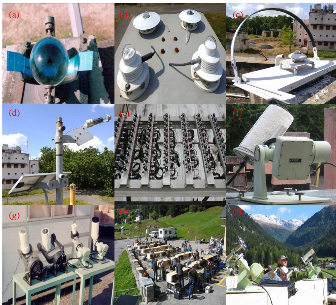
Figs. 7(a-i). Campbell Stoke duration of bright sunshine recorder, (b) Thermoelectric pyranometer, pyrgeometer, UV A radiometer, UV B radiometer, (c) Diffuse Shading ring with Pyranometer (d) Electronic sunshine duration sensor (e) Pyranometer sensors for outdoor calibration (f) Cavity Radiometer (g) Four Cavity Radiometers (h) IPC 2015 at Davos, Switzerland (i) IMD Cavity Radiometer at IPC 2015
