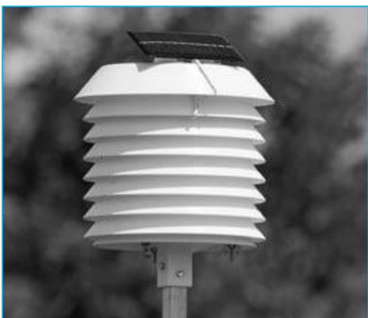
Fig. 3. Louvred screen in an automatic weather station
