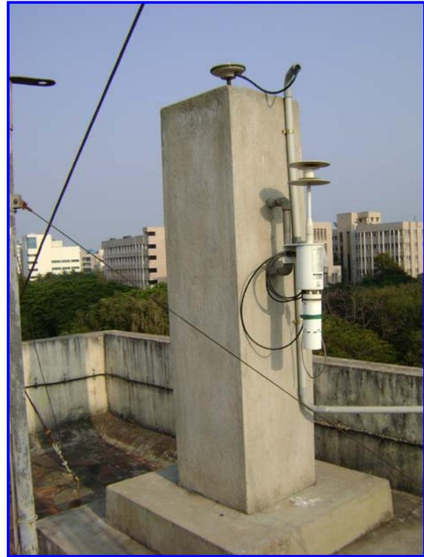
**Fig. 1.** Photograph of GPS equipment Leica GPS Spider with Met3A meteorological sensors installed at Chennai (Nungambakkam)
