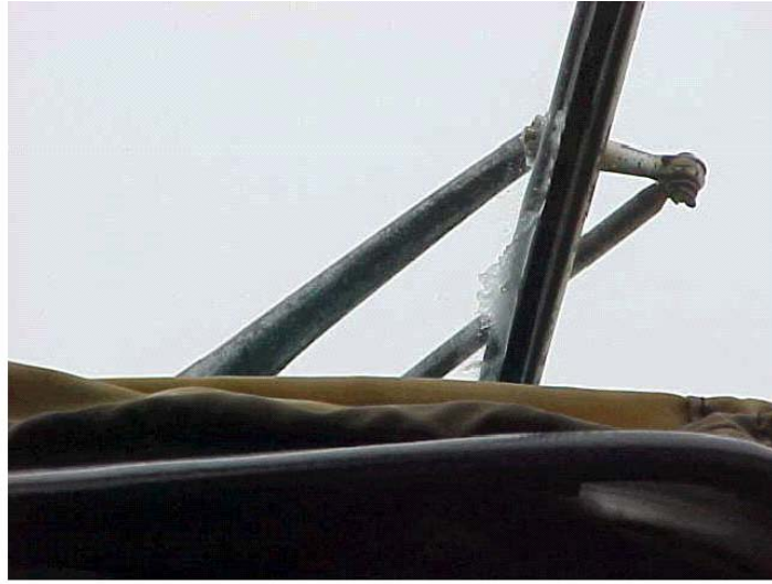
PHOTOGRAPH OF ICING ON COCKPIT WINDOW Date/Time : 26 Jun 02/1302 IST Altitude : 20000 feet Location : BETWEEN POINT A AND GOA (16.46/71.58)
