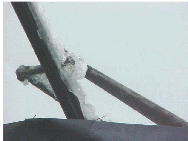
PHOTOGRAPH OF ICING ON COCKPIT WINDOW Date/Time : 18 Jun 2002/1313 IST Altitude : 20000 Feet Location: BETWEEN POINT A AND GOA (16.24/72.27)
