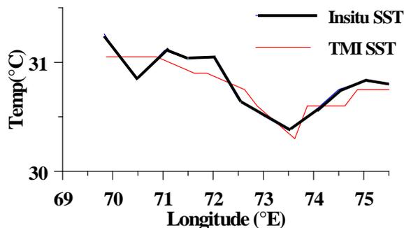
Fig. 1. Comparison of sea truth SST and TMI SST
