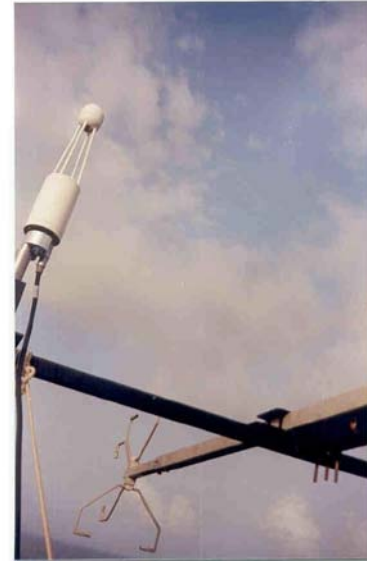
Fig. 2. Licor – 7500 H 2 O and CO 2 analyser (Left) on the tower at 5m agl at NCAOR, Goa
