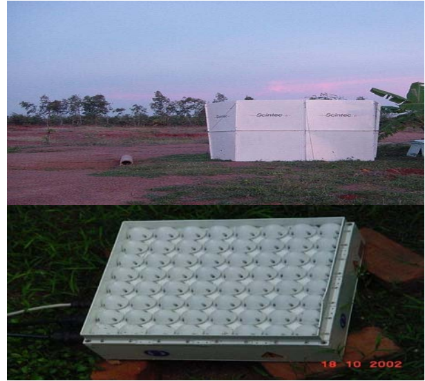
Fig. 2. Mini-Sodar antenna and enclosure
